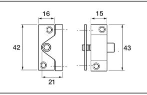
• Lock is surface fixed onto the window section, locking into the fixed frame by use of the key
