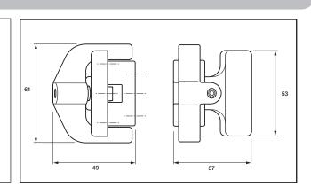
• Lock for surface fixing onto the window section which is locked around the frame fixed staple by use of the key
