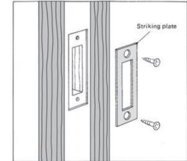
• Screw striking plate to frame and mark around outside shape and around bolt hole. Remove plate and chisel out bolt hole slightly oversize to a depth of 13mm. Chisel out shape of striking plate to a depth of 3mm until the plate is flush with the frame. Re-fit striking plate.
