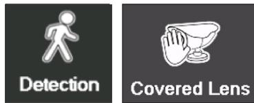
From the Main Menu, hover over 'Detection' and then move mouse over 'Covered Lens' and left click to select. This function helps detect any deliberate covering of the camera lens to obstruct recording. To enable covered lens detection, select the channel/camera you wish to activate then check the Enable box next to Channel.
