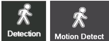
From the Main Menu, hover over 'Detection' and then move mouse over 'Motion Detect' and left click to select. This option allows you to set the DVR to record when motion is detected in selected areas i.e. window, doorway, gate or driveway.
