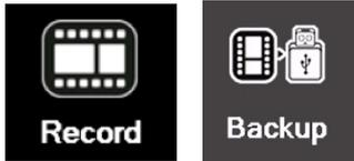
From the Main Menu, hover over 'Record' and then move mouse over 'Backup' and left click to select. This option allows you to back up your video recording onto a USB Flash Drive.
