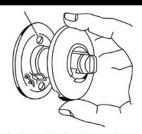
Detach the inner plate from the round cover of the inside knob side, fasten it to the lock with machine screws supplied and tighten machine screws, replace the round cover.
