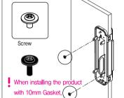
Secure the plate with the 2 plate
