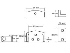
• Surface fixed lock that swings over a frame fixed striking plate
