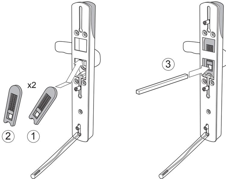
Slide the lug up or down to align with the holes in the door.
