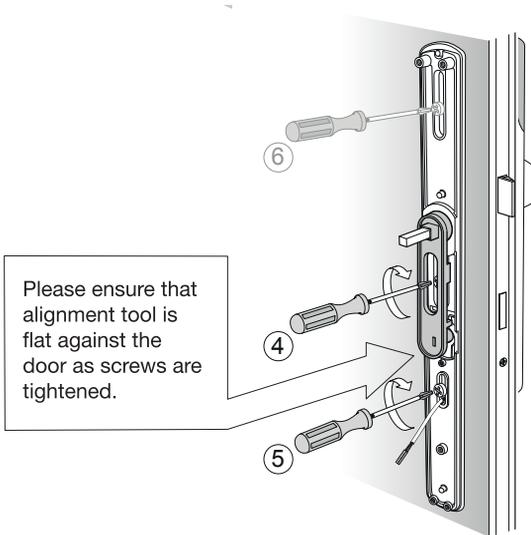
Please ensure that alignment tool is flat against the door as screws are tightened.
