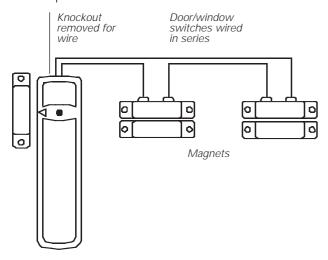
It is possible to use a single pair of multiple door/window contacts with a detector if you experience problems fitting the main unit to the door frame.
