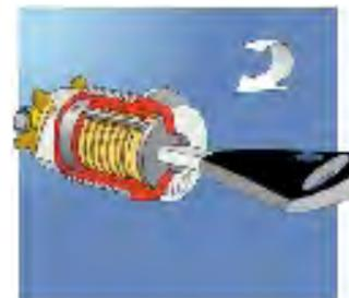
3. The locking bar is now able to enter the slot. The key can then be turned further to operate the lock.
