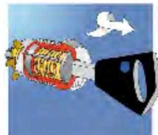
4. To withdraw the key, it is turned in the reverse direction until it stops. This automatically scrambles the detainer disc combination. The key meets no resistance when being withdrawn from the cylinder.
