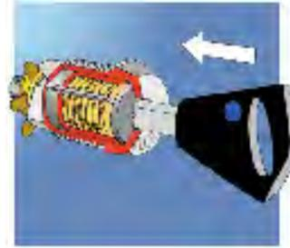
1. The key meets no resistance when it is inserted into the keyway. There are no spring loaded parts to wear out.
