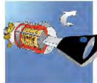
2. The correct key, when fully inserted and turned, allows rotation of the detainer discs to the correct position.
